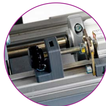
Adjustment knob for easy tuning of the position of the Y blade set on the machine.
